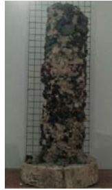
Figure 5 Deformed shape of natural aggregate granular column
