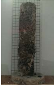
Figure 4 Deformed shape of cupola slag granular column
